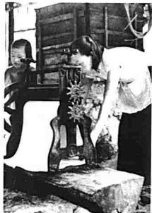
Fig. 234 A Fuzhou mother and her daughter putting rubber sheets through the rollers of a manually-operated mangle. (Photo: Hedda Morrison)
