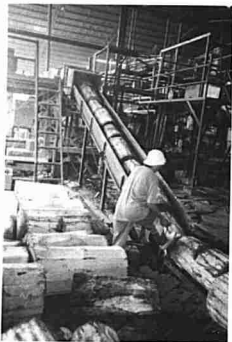
Fig. 349 Logs of Sago are being carried by conveyor-belt to the grating machine where the grated sago is mixed with water and sieved to extract the sago powder.
